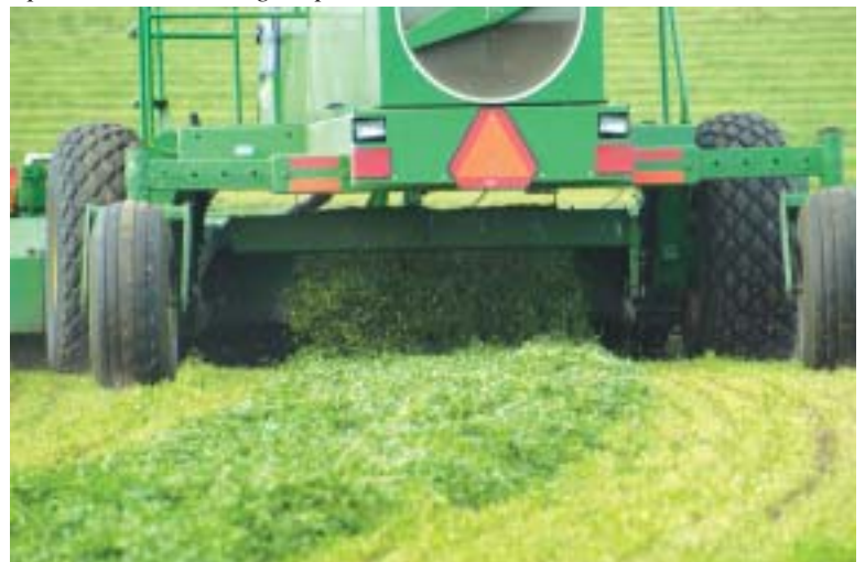
Windrow being layed down by John Deere 4995 with 994 header at 10 mph in wet 4th cutting crop.
