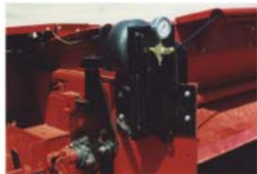
Airbags are filled easily using a pump or compressor much like filling a tire. The gage informs the user of the actual air pressure in the system, allowing him to adjust the pressure to the crop being cut.
