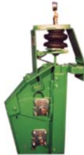
Typical mounting for airbag system on the Super Conditioner. Air pressure pushes down on the bearing plate, creating linear pressure between the conditioner rolls.
